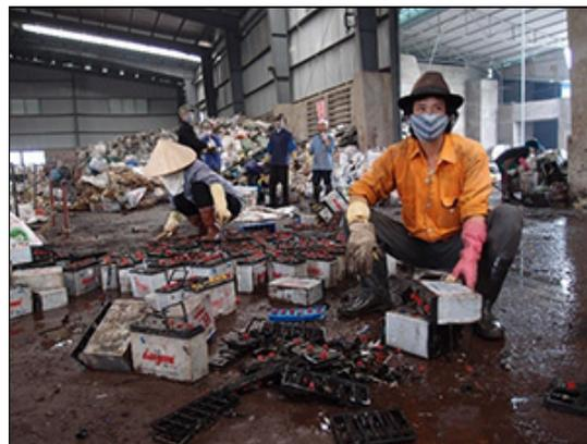
Workers in a lead battery recycling facility outside Dong Mai village break batteries apart and separate metal and plastic components.
