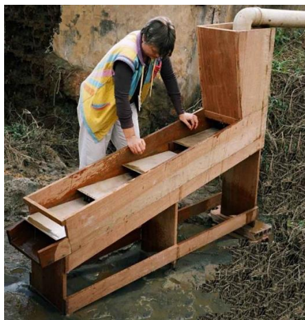
Figure 2 Silver-Covered Copper Plates in a Cascade Arrangement
