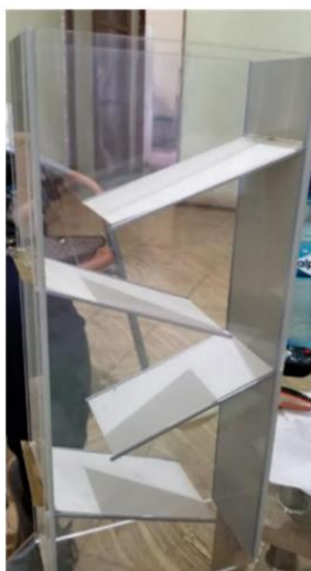
Figure 3 Silver-Covered Copper Plates in a ZigZag Arrangement
