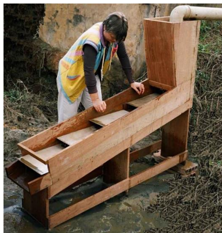
Figure 2 Silver-Covered Copper Plates in a Cascade Arrangement
