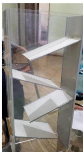
Figure 3 Silver-Covered Copper Plates in a ZigZag Arrangement
