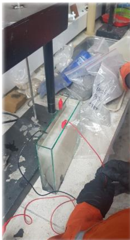
Figure 7. Assembly of the electrolysis process
