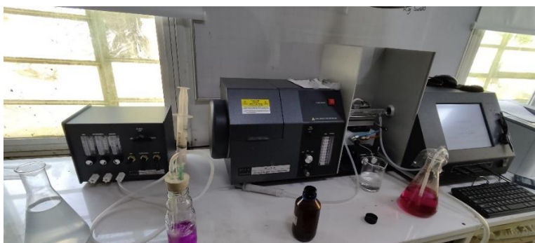
Figure 15. Hg readings through cold vapor atomic absorption.
