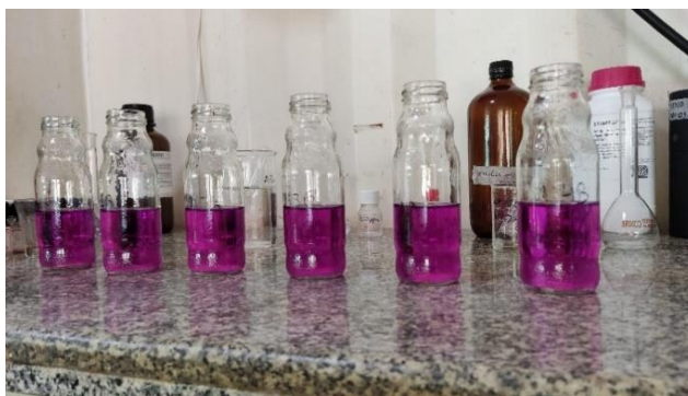
Figure 14. Sample preparation for atomic absorption spectrophotometry reading.
