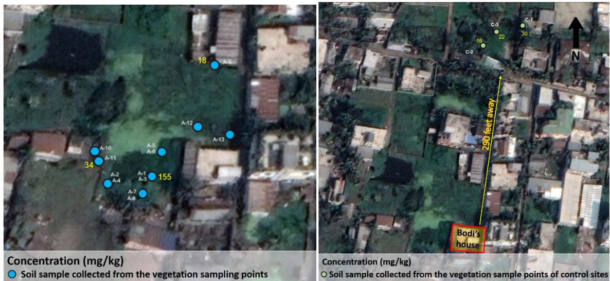
Figure 15: Shows Pb concentration of soil samples collected within 50 m of ULAB recycling site and control site.
