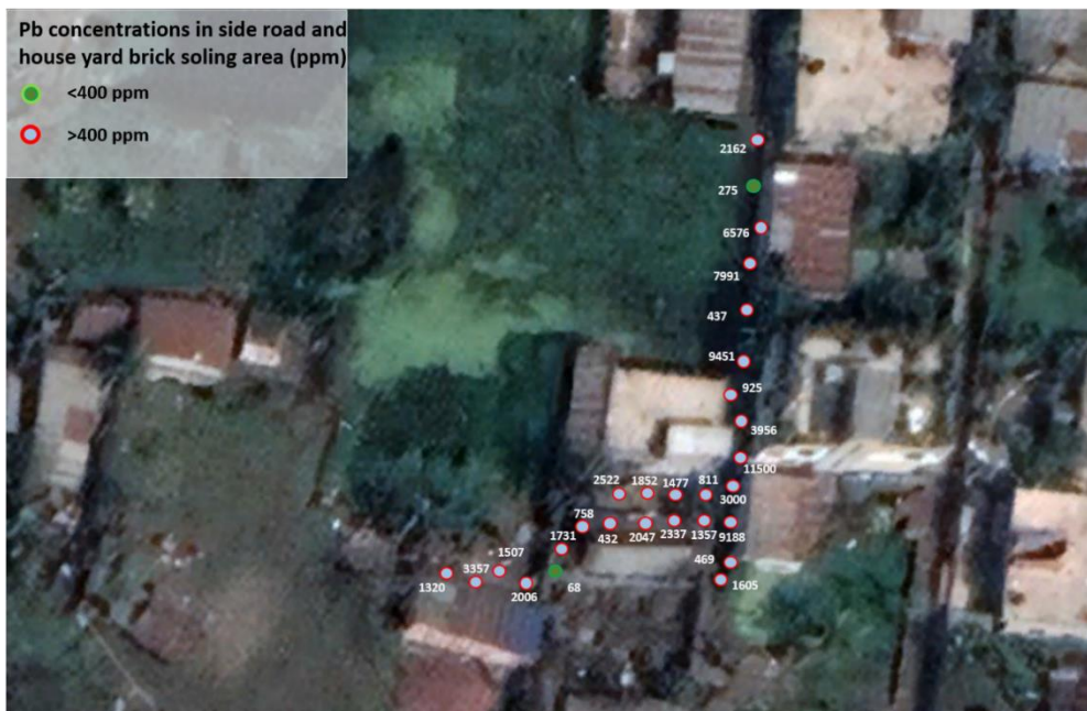
Figure 31: Pb concentrations in the brick soling road and house yard areas after soil scraping.
