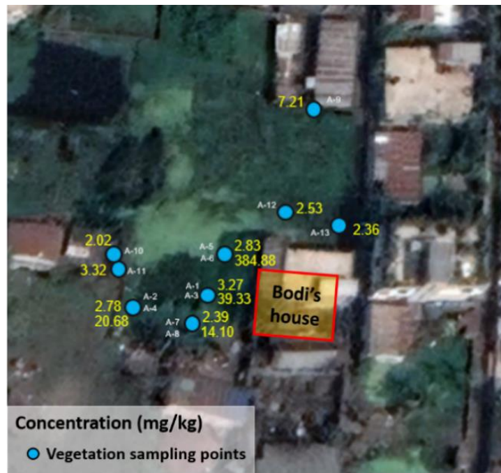
Figure 14: Shows Pb concentration of vegetable samples collected within 50 m of ULAB recycling site and control site.
