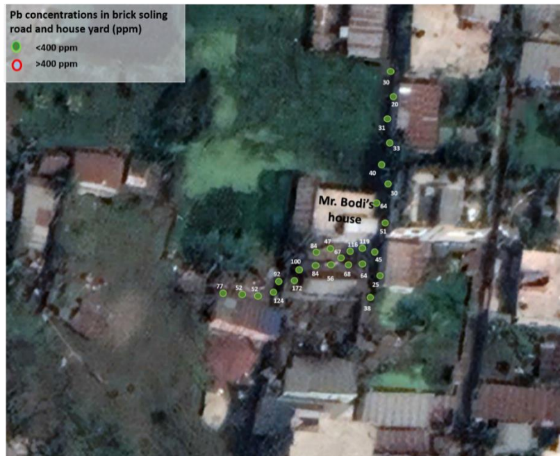
Figure 34: Map showing lead concentration of yard, road areas after concrete work
