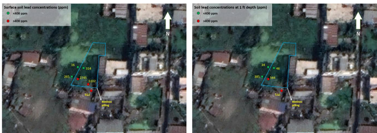
Figure 20: Pb concentrations of surface and 1 ft depth soil samples from inside and outside of the bamboo piling area of the West dumping site.
