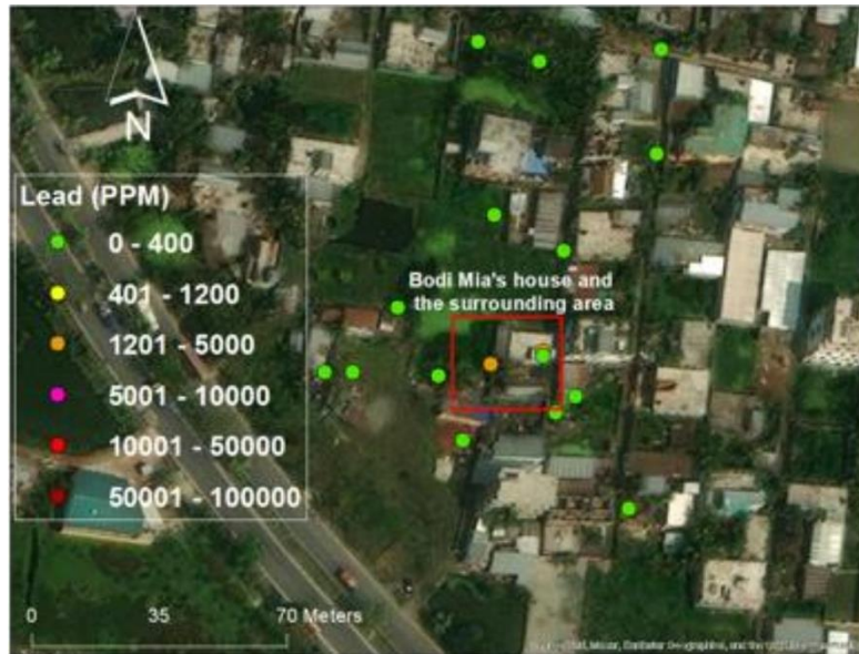
Figure 2: Lead concentration map showing the extent of XRF measurement (source: PSA report).
