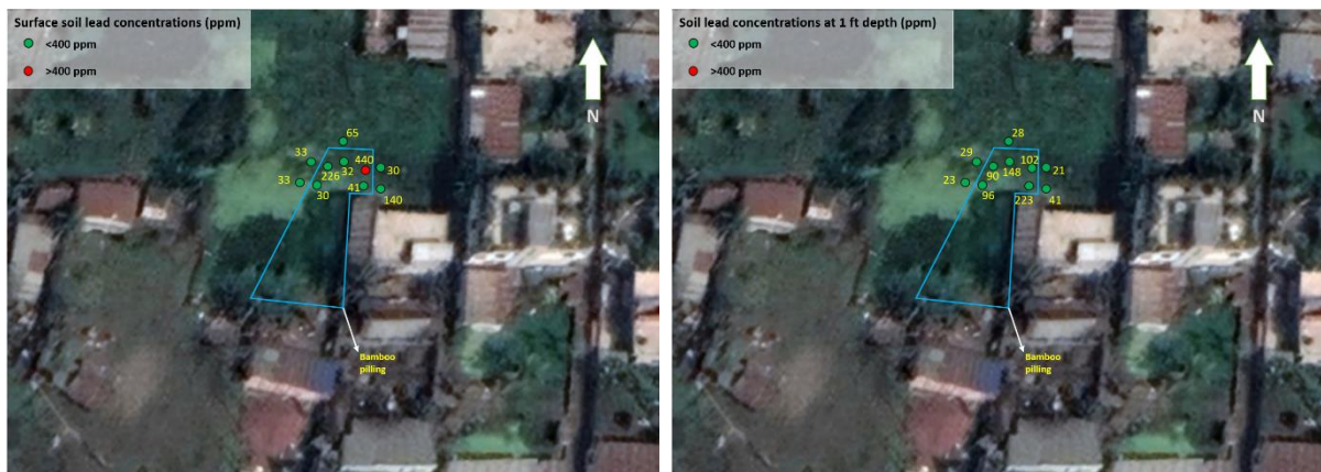
Figure 19: Pb concentrations of surface and 1 ft depth soil samples from inside and outside of the bamboo piling area of the North dumping site
