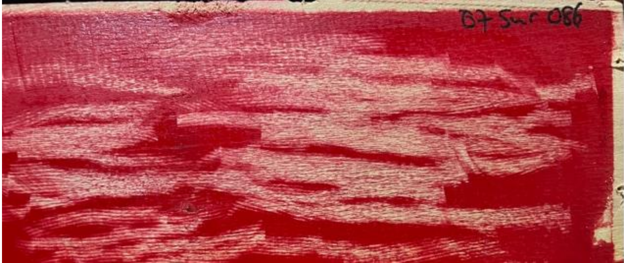
Sample 07SUR086 from Indonesia demonstrating thin red paint scraped from a wooden toy for laboratory testing.
