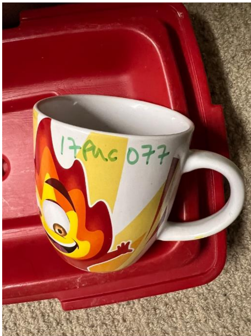
Sample 17PUC077 from Peru with XRF lead at ND,17 in the interior white portion and 12,000 ppm in the decorative exterior portion.
