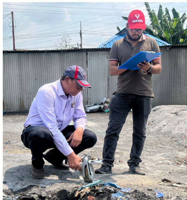
An investigator uses an X-Ray Fluorescence analyzer to test the ground outside a home in Bangladesh.
