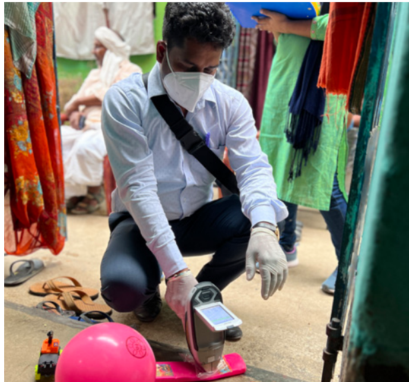
A Pure Earth investigator uses an XRF (X-Ray Fluorescence) analyzer to test a child's toy in a home in India.
