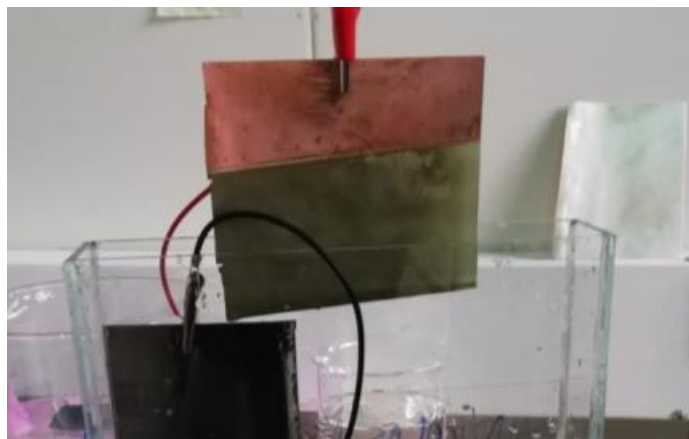
Figure 4. Silver plating on the copper plates with electric potential. Source: Pure Earth.
