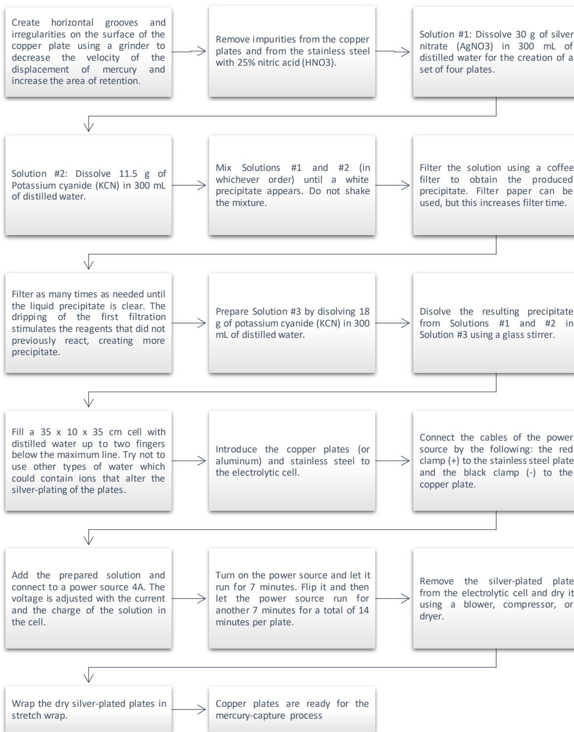
Figure 3. Procedure for the electrochemical plating of the copper plates. Source: Pure Earth.
