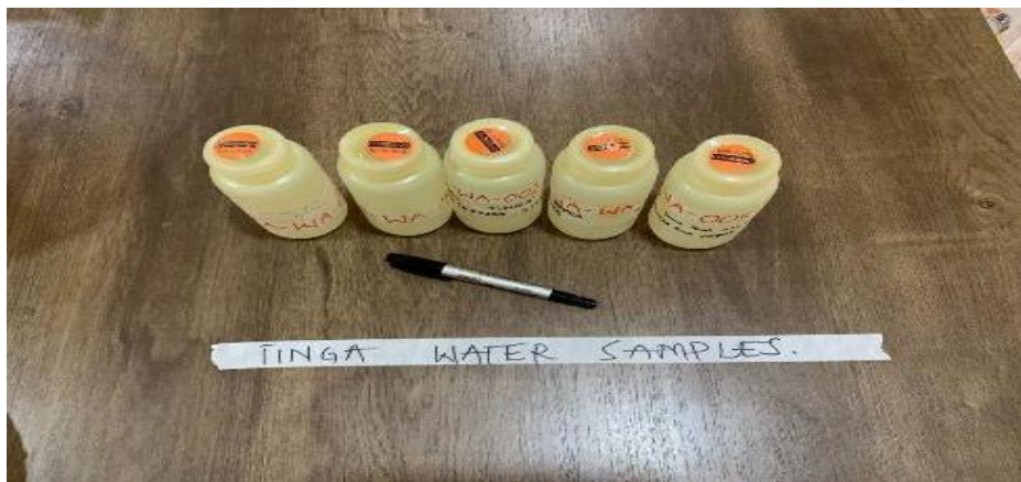
Figure 3.6: Water Samples in Bottles Filled with Nitric Acid
